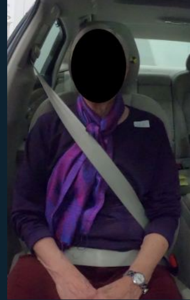
Shoulder belt positioned over the mid portion of the shoulder
